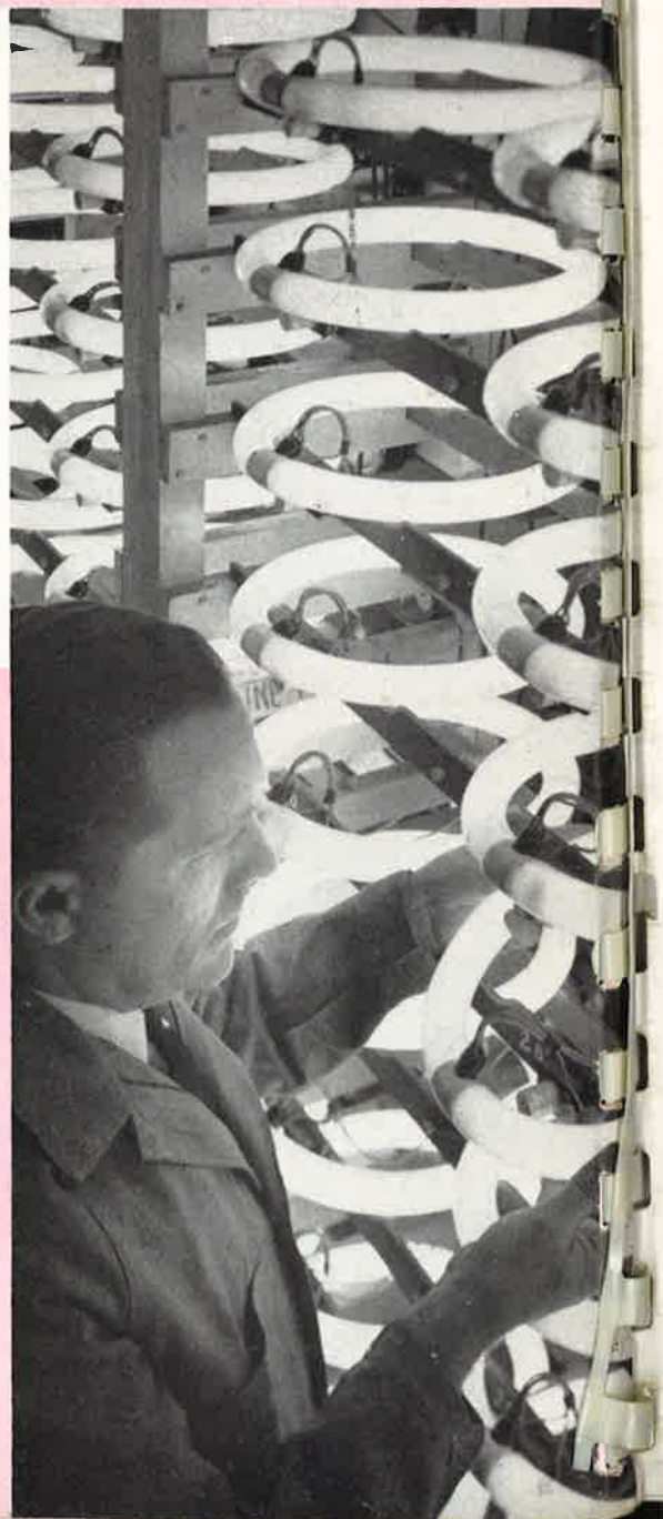
QUALITY CONTROL is as important in the continuing improvement of lamp manufacture as it is in lighting application. Equipment above makes possible 99.998% purity in the drop of mercury which goes into each fluorescent lamp.
