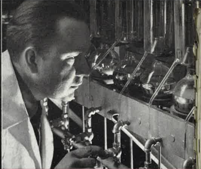
QUALITY CONTROL is as important in the continuing improvement of lamp manufacture as it is in lighting application. Equipment above makes possible 99.998% purity in the drop of mercury which goes into each fluorescent lamp.
