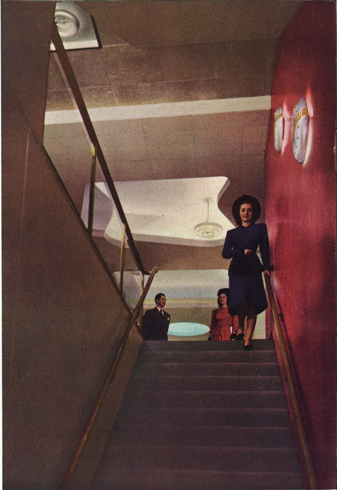
ARCHITECTURAL HANDLING OF THE STAIRWAYS was planned to give a feeling of unity and spaciousness and to invite the visitor from the main floor to the auditorium above or the ground floor below. Plaques of perforated metal shielding Circline lamps add decorative spots and provide illumination for stairs.
