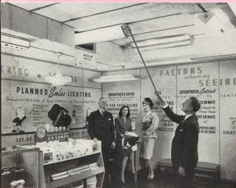
NO FOREST of fixtures here. A. F. Loewe demonstrates an idea for showing one fixture at a time. Fixtures pull out of a wall soffit on tracks. Customer can choose better when ceiling is not cluttered with a bank of varying sizes and shapes of fixtures.
